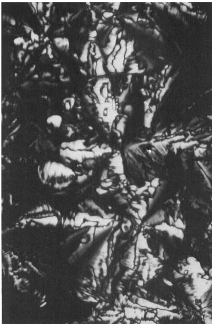
Figure 2. Photomicrograph of the mesophase of 1e obtained by heating, viewed between crossed polarizers ( T=74^{\circ}\text{C} ).
